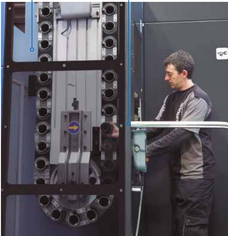
Sliding shutters to ease tool loading / unloading
